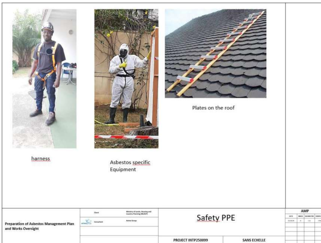
Figure 13. Safety PPE required
